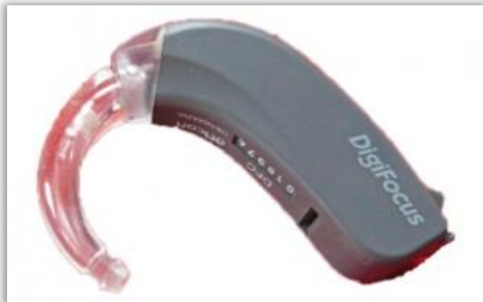
Figure 10: Oticon Digi Focus Compact from 1996 (Bauman, 2015)
